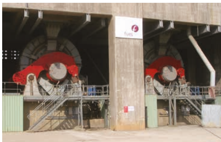
The combination of two identical FCB Horomill® grinding units operating simultaneously along with a large-sized FCB TSV™ Classifier.
