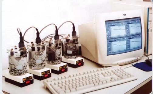
The CAA is a computer based, automated instrument that provides independent, simultaneous measurement of the activity of up to four samples of carbon.
