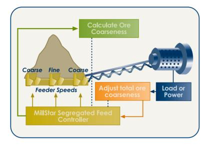
MillStar's Segregated Ore Feed Controller is designed to:
