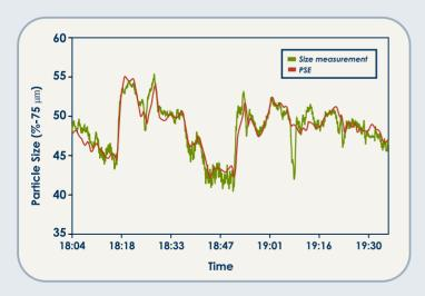
The graph above shows how well the PSE tracks the real particle size measurement. Note how it can be used to eliminate spikes and noise in the measurement.
