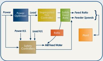
With optimising the mill power and preventing mill overloads significant increases in throughput of between 6 and 16 % have been achieved.
