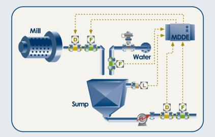
The Mill Discharge Density Estimator estimates the mill discharge density and flow using dynamic volume and mass balances. An energy balance can optionally be performed to enhance the accuracy of the estimate. Grinding efficiency is highly dependent on the viscosity of the material within the mill, which correlates closely with the density. The calculated density can therefore be controlled by changing the amount of water added to the mill, to ensure optimum grinding.
